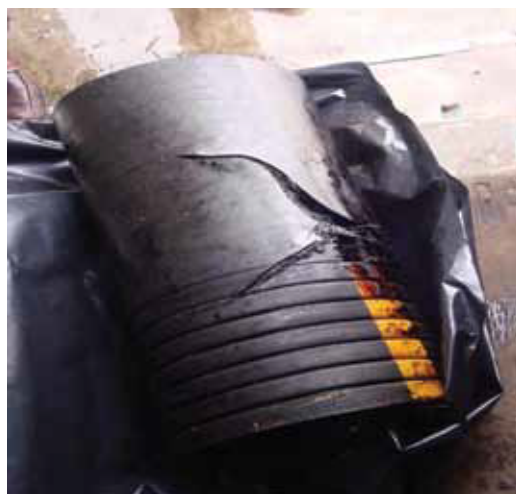
^ Cropped section of damaged bunker hose
