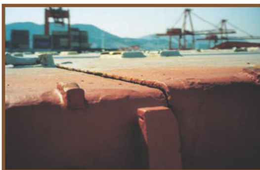
When closed the top of a hatch panel should be in line with the next panel.
