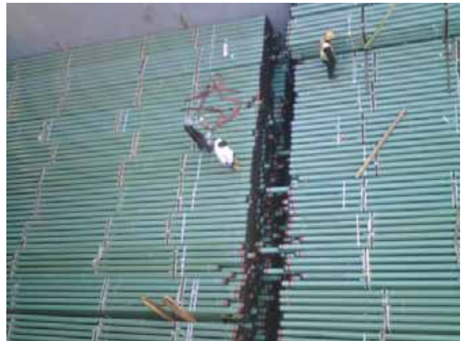
Bundles of coated pipes are stowed with vertical chocking.
