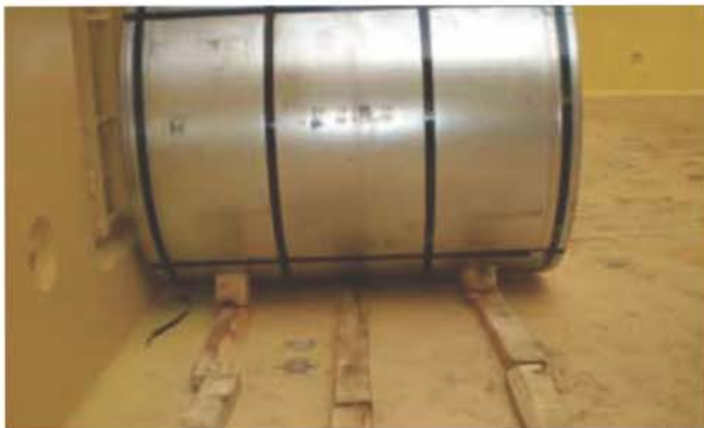
Coils wedged in position.
