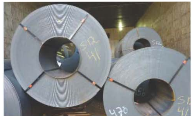
This key coil appears to exceed the 60% rule.
