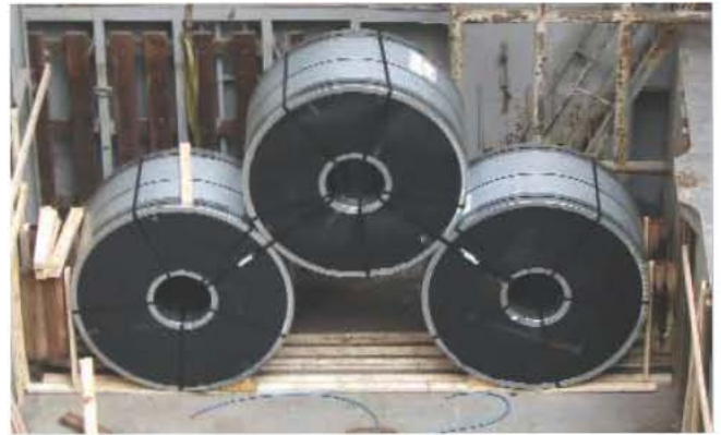
Coils correctly stowed with dunnage, wedges and a key coil.
