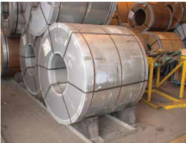
Coil prior to stowage correctly wedged.
