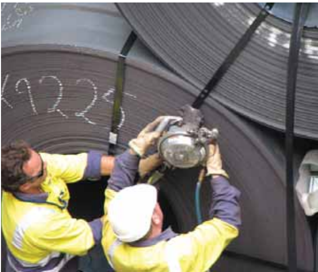
Steel bands are pneumatically tightened.
