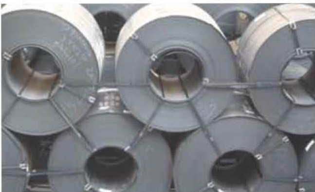
Coils stowed and lashed together with steel bands.
