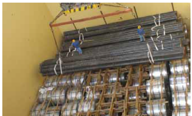
Pipes loaded on top of coils need to be securely lashed to prevent movement. Dunnage has been placed between the pipes and the longitudinal bulkhead.
