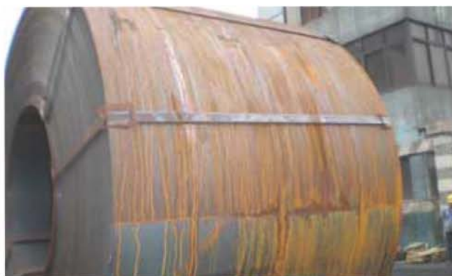
Condition of coils at discharge port - rusted.
