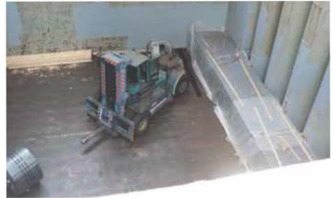
Coils being stowed by a forklift fitted with a single round tine.
