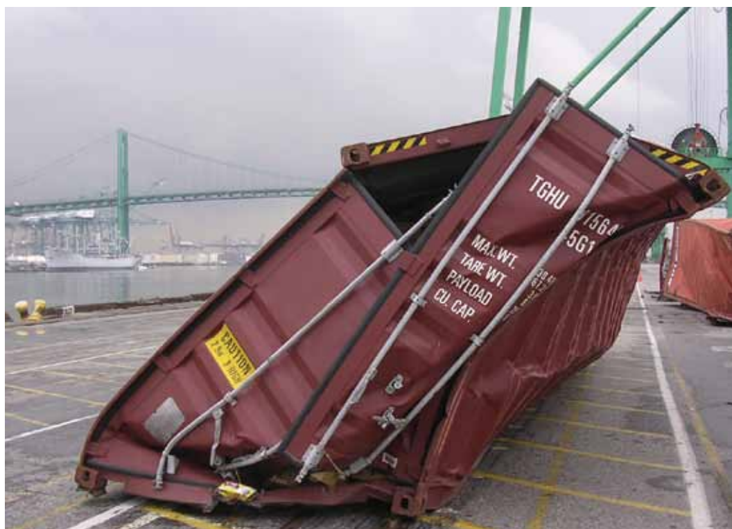
^ Collapsed container – crush damage
