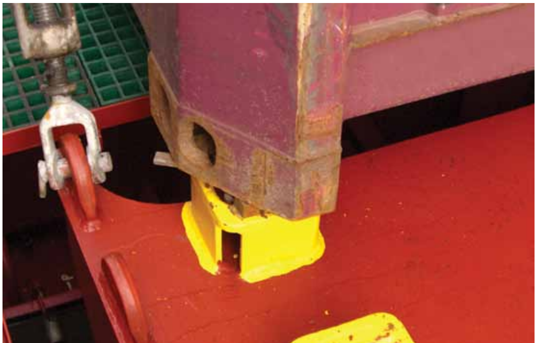
^ Corner casting arrangement for a Euro container
