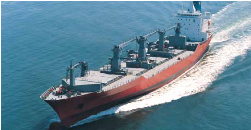
^ Multi-purpose general cargo ship with capacity to carry containers on deck
