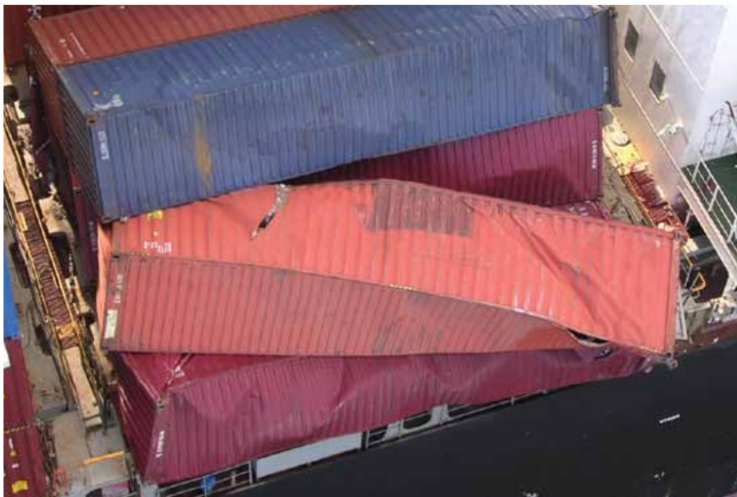
^ Lashing failure causing container loss
