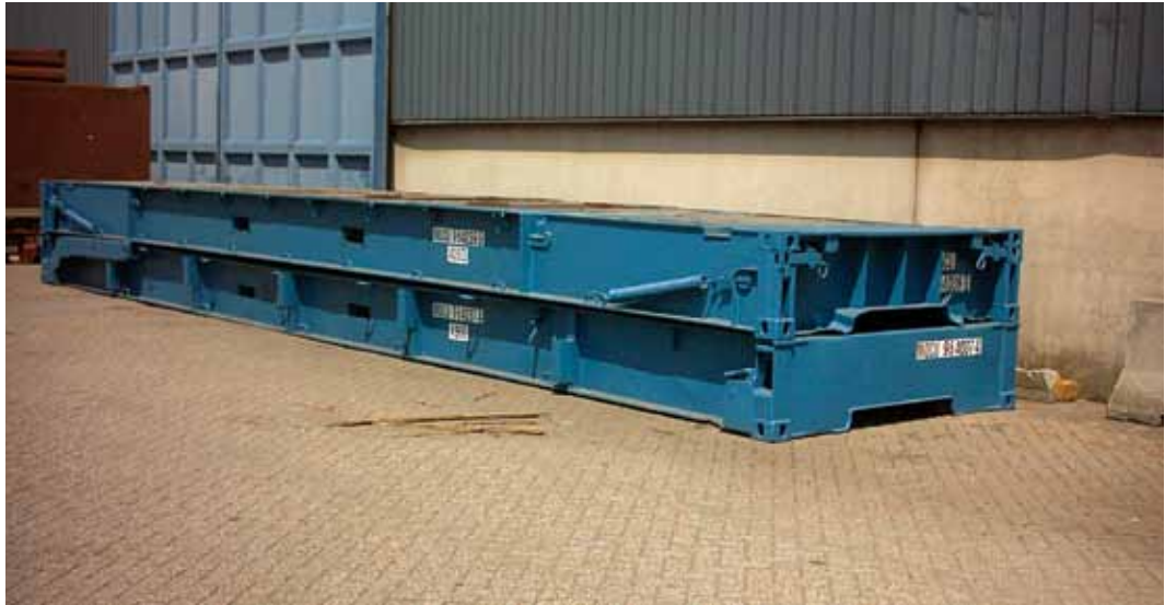
^ Two flat racks over stowed
