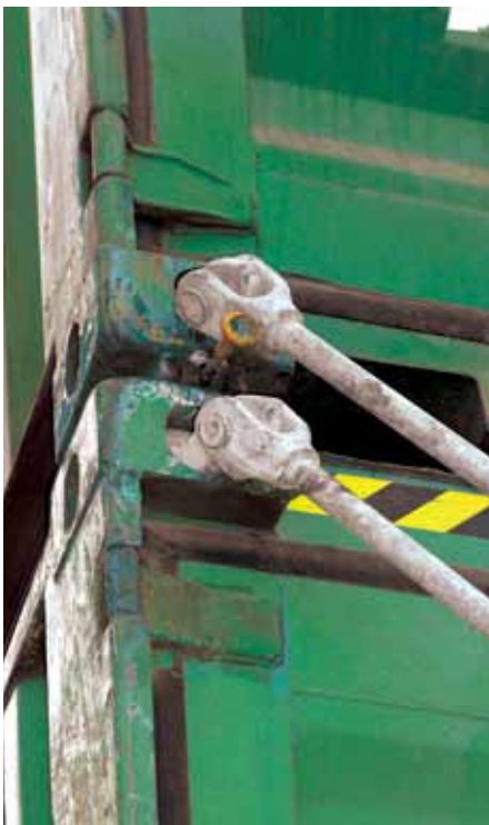
^ Securing with parallel lashing rods and semi-automatic twistlock
