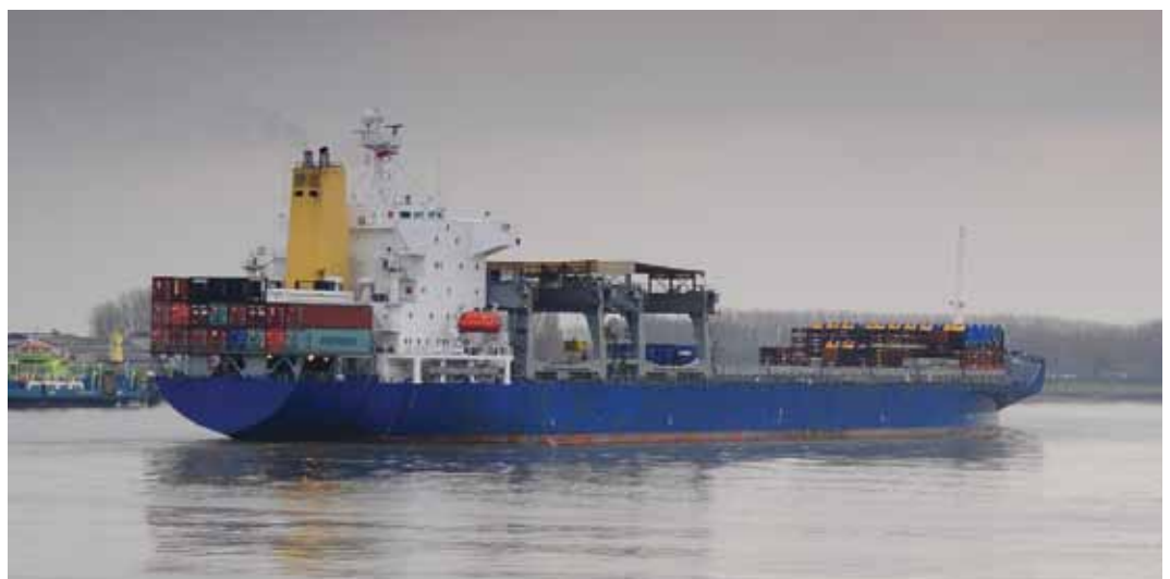
^ Typical arrangement for con-bulker with gantry crane
