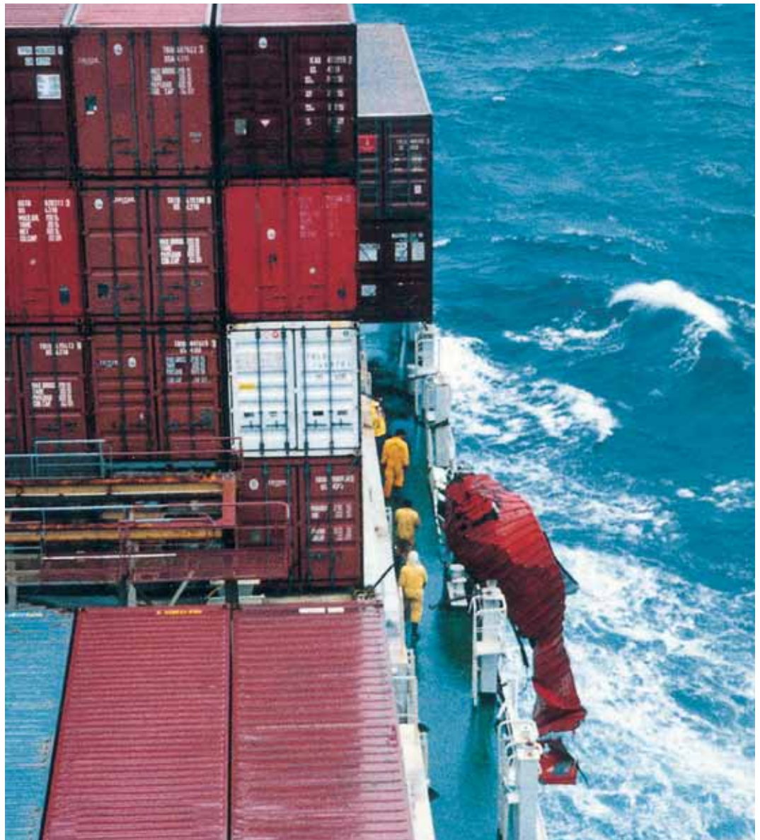
^ Outboard container damaged by heavy sea
