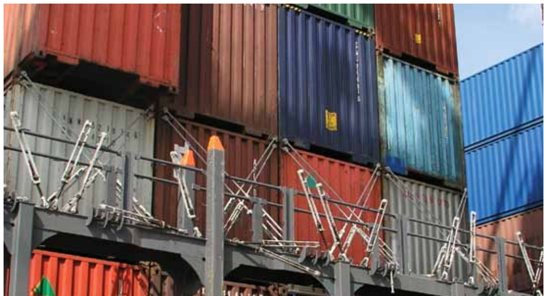
^ Do not lash to the overhanging end of a 45-foot container
