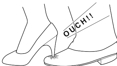
Figure 54.2b: The heel of the shoe is exerting a point loading of 1,200 t/m 2 .
