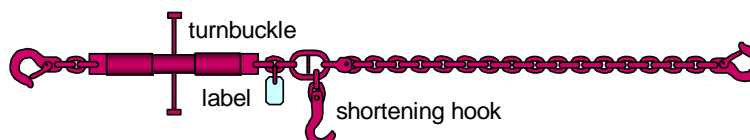
Figure 7.18 Standard chain lashing with shortening hook
