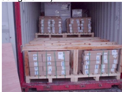
Figure 7.2 Timber temporary floor
