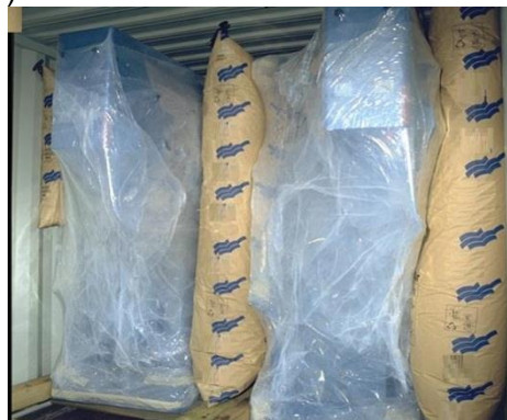
Figure 7.10 Irregular shaped packages blocked with dunnage bags
