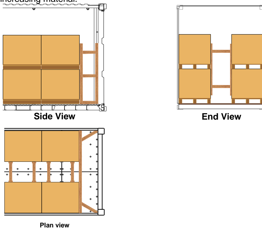
Figure 7.32 Blocking in a strong boundary CTU
