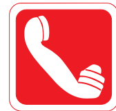
Emergency fire telephone
