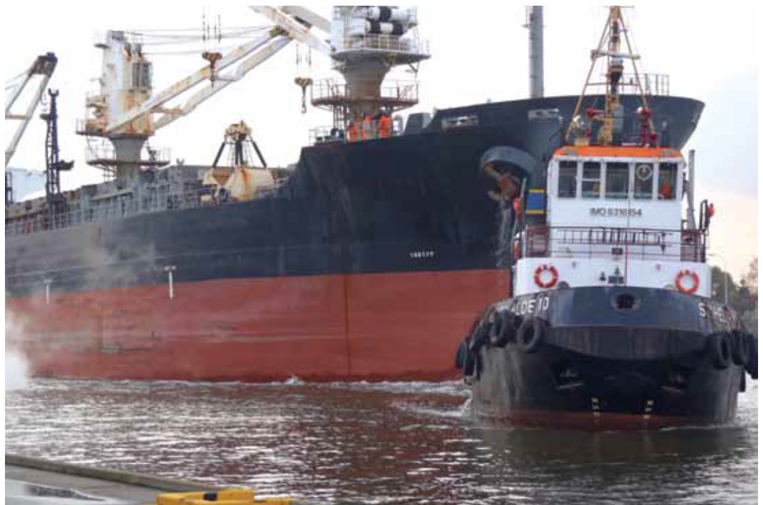
^ Using the tug to bring the ship close to the berth
